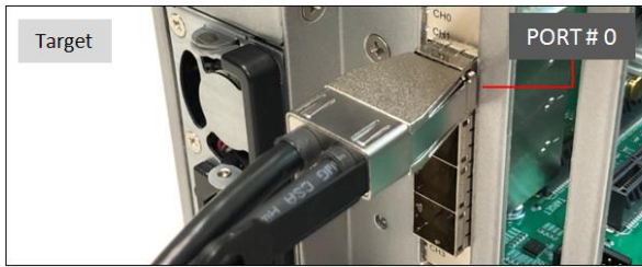
Photo A1: Cable is connected on the Target card PORT # 0. The other end of the cable is connected on the Host card PORT # 1
